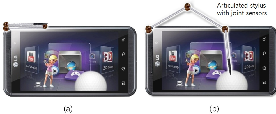
FIGURE 1. 3D interaction on a stereoscopic phone using an articulated stylus with joint sensors for 3D position tracking. The stylus can be folded for easy stow away (left).
