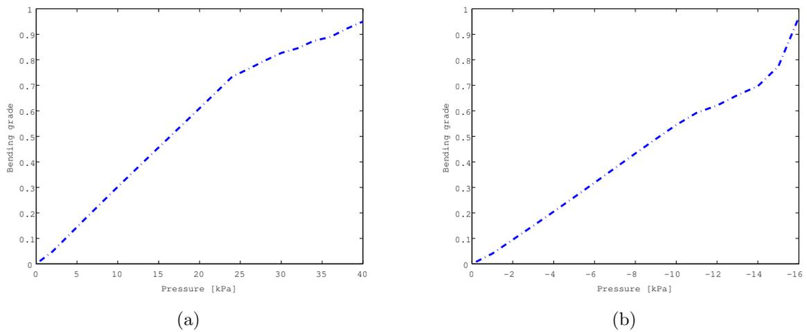
FIGURE 9. (a) The identified bending grade  $\rho$  in different positive pressures; (b) the identified bending grade  $\rho$  in different negative pressures
