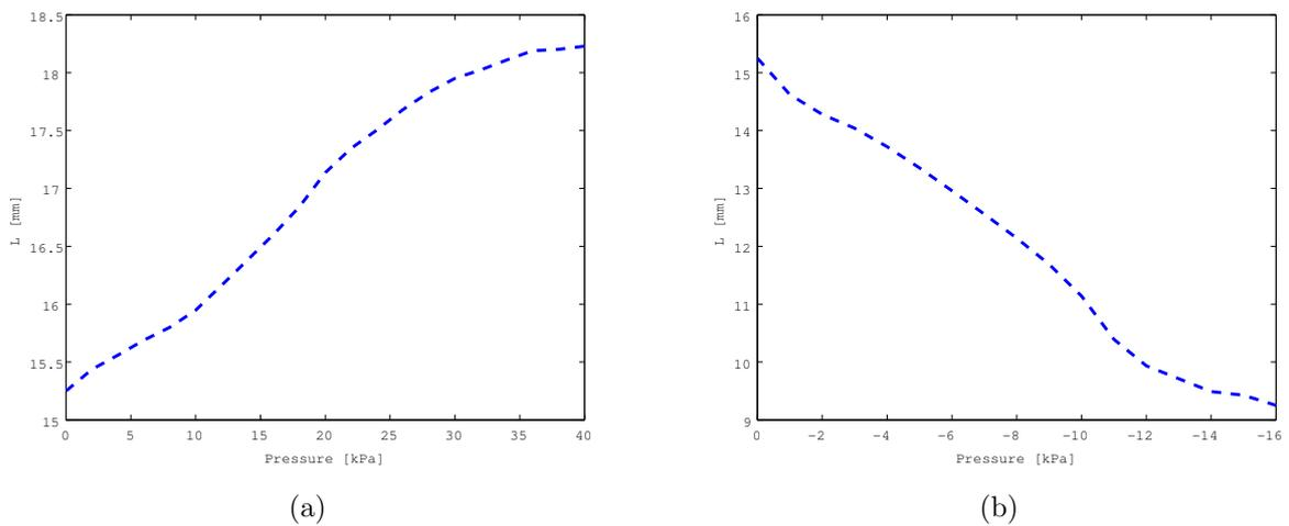
FIGURE 10. (a) The identified arc length  $L$  in different positive pressures; (b) the identified arc length  $L$  in different negative pressures
