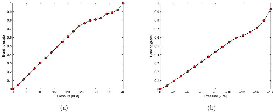
FIGURE 6. (a) The calculated bending grade  $\rho$  in different positive pressures; (b) the calculated bending grade  $\rho$  in different negative pressures
