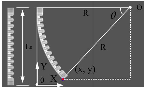
FIGURE 3. Calculation of the position based on bending grade and arc length
