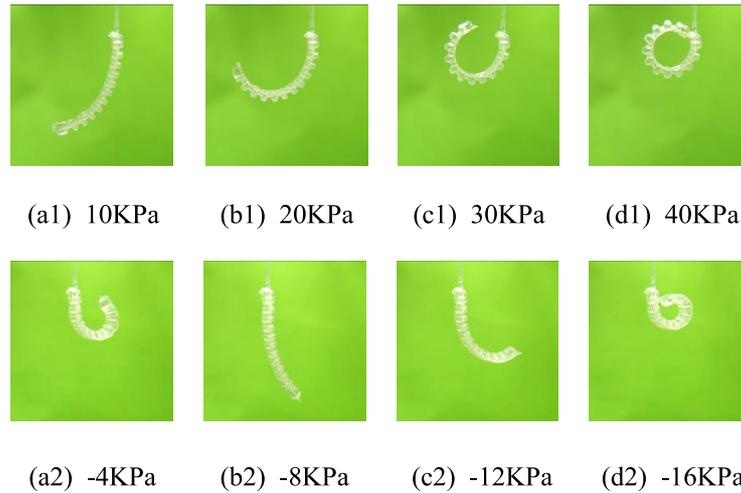
FIGURE 1. Bidirectional motion in different positive and negative pressures
