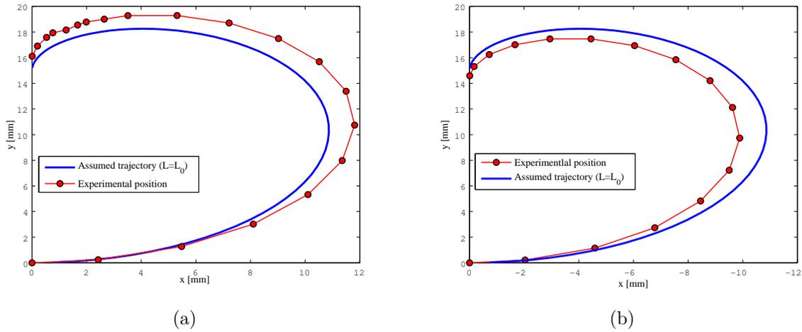
FIGURE 5. (a) The measured position  $(x, y)$  in different positive pressures; (b) the measured position  $(x, y)$  in different negative pressures
