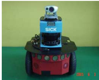
FIGURE 12. Pioneer3-DX mobile robot with laser range finder
