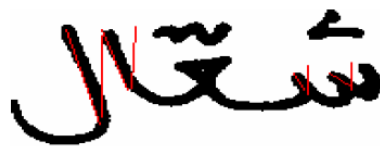
FIGURE 6. Locally angle computation for slant normalization
