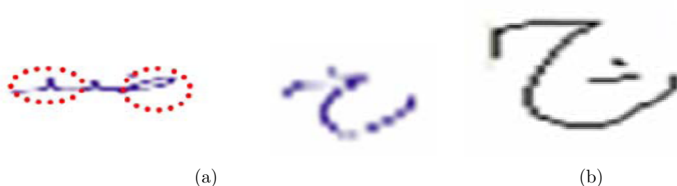
FIGURE 4. (a) Missing points due to fast speed of writing; (b) smoothed and interpolated stroke
