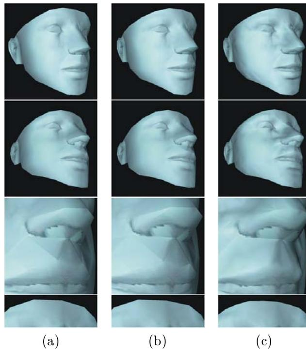
FIGURE 11. (a) Original facial model, (b) improved result and (c) smoothing
