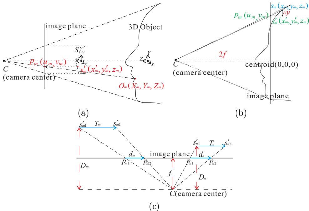
FIGURE 3. (a) Point  $p_m$  in the image plane represents the 2D projection point of both the 3D reconstructed point  $s'_m$  in the orthographic model and the 3D object point  $O_m$  in the perspective model; (b) difference  $\Delta y$  between the reconstruction results in the  $y$ -axis direction obtained from the orthographic and the perspective model, respectively; (c) determining the camera focal length  $f$
