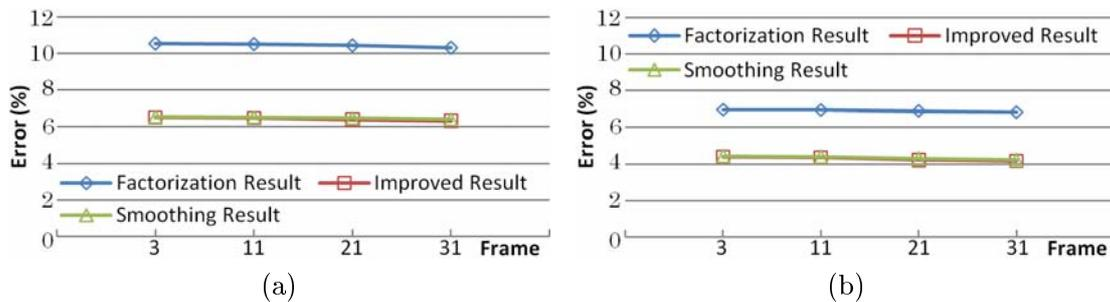
FIGURE 8. Comparison of reconstruction errors of different reconstruction results: (a) at distance  $d$  of 35 units ( $\Delta d/d \approx 1/5$ ) and (b) at distance  $d$  of 50 units ( $\Delta d/d \approx 1/7$ )
