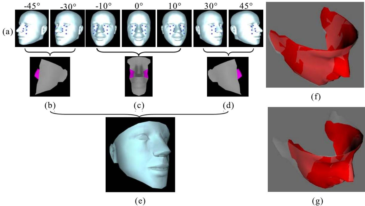
FIGURE 5. (a) Sequence of facial images under different pan-rotation angles; (b)-(d) improved results in which the purple regions denote overlapping regions (the dots shown in (a)); (e) registered result; (f) and (g) registration results obtained using different overlapping regions
