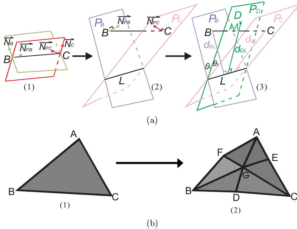
FIGURE 4. (a) Example of smoothing method and (b) smoothing result obtained for each polygon in 3D space
