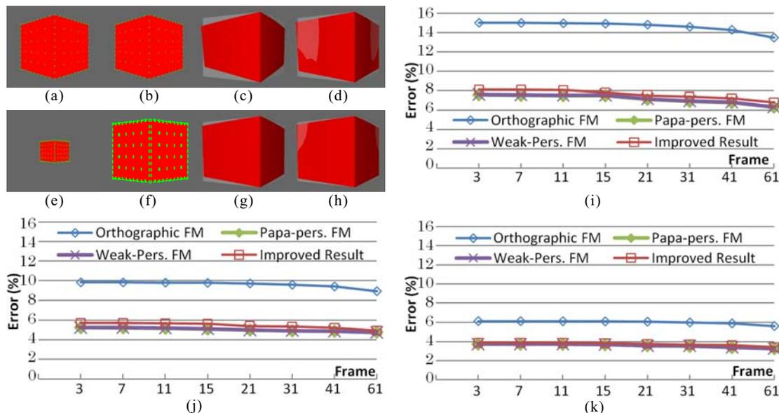
FIGURE 6. (a)-(d) and (e)-(h) Reconstruction results obtained when using  $\Delta d/d$  ratios of  $1/3$  and  $1/7$ , respectively. (a) and (e) Original images, (b) and (f) close-up view of boxes, (c) and (g) factorization results, and (d) and (h) improved results. (i)-(k) are the estimation errors of reconstructed boxes given  $\Delta d/d$  equal to  $1/3$ ,  $1/5$  and  $1/7$ , respectively.
