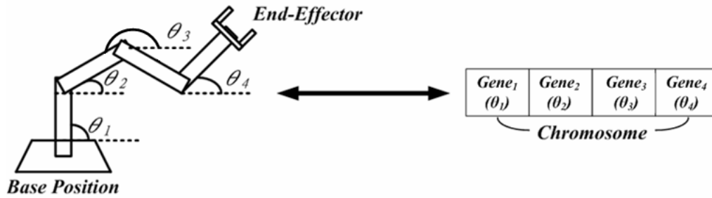
FIGURE 5. Configuration of a manipulator represented as a chromosome with the genes representing the joint angles
