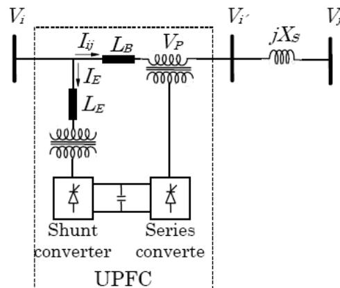
FIGURE 1. Basic schematic diagram of UPFC
