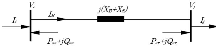
FIGURE 2. The power injection model of UPFC
