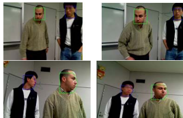
FIGURE 5. Top 2: An example for human face tracking for two persons: (left) Frame 306, (right) Frame 400, Bottom 2: human face tracking in different orientations of the face: (left) Frame 323, (right) Frame 390
