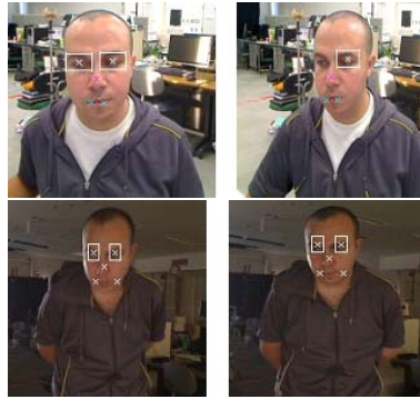
FIGURE 7. Top: Video sequence one, shows a person tracked with different rotation: (left) Frame 193, (right) Frame 198, Bottom 2: Tracking under different light conditions movement: (left) Frame 59, (right) Frame 243
