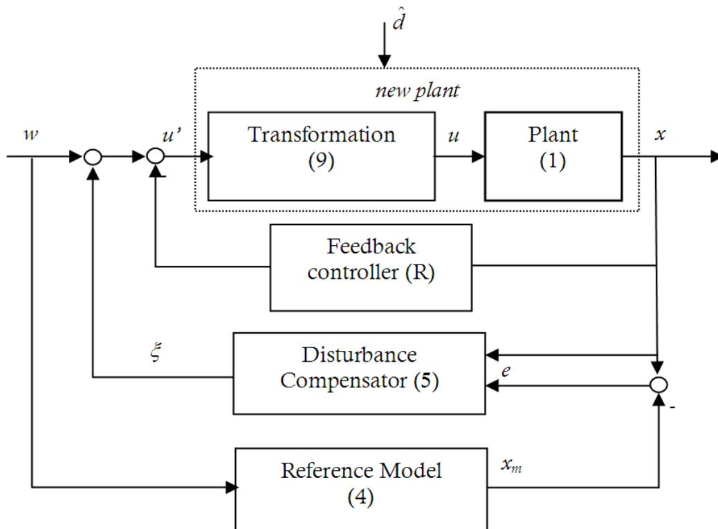
FIGURE 1. The structure of the linear adaptive GAS controller
