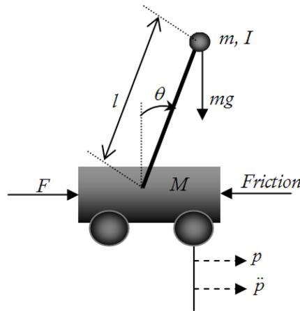
FIGURE 6. Inverted cart pendulum system and force diagram
