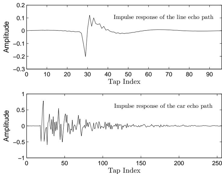
FIGURE 6. Impulse responses of the line and car echo paths
