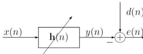
FIGURE 1. Prototypical adaptive filter setup
