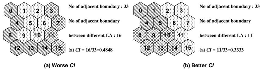
FIGURE 1. Configurations of  $LA_1$  and  $LA_2$
