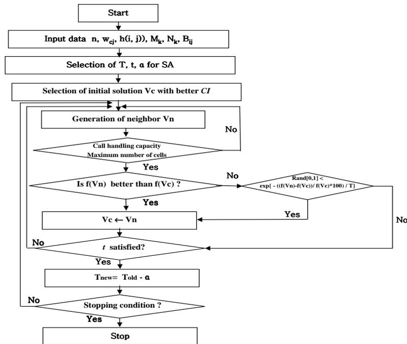
FIGURE 2. Flowchart of SA with compact index
