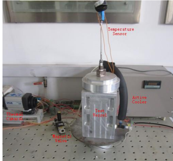
FIGURE 1. Leak diagnosis and localization apparatus
