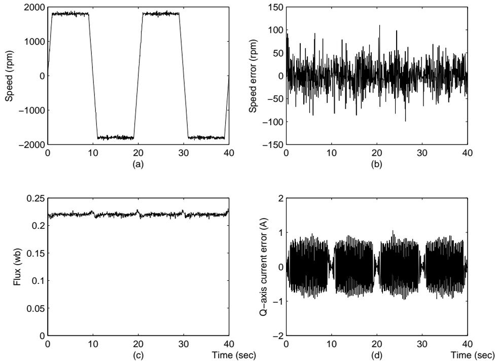
FIGURE 9. Simulation results corresponding to the CM flux observer on  $\omega_{rm}^* = 1800$  rpm: (a) speed response, (b) speed error, (c) rotor flux, (d)  $q$ -axis current error
