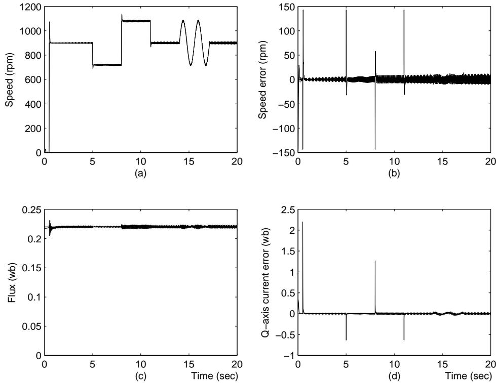
FIGURE 5. Simulation results corresponding to the SM flux observer: (a) speed response, (b) speed error, (c) rotor flux, (d)  $q$ -axis current error
