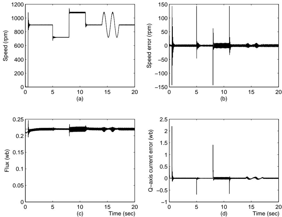
FIGURE 4. Simulation results corresponding to the CM flux observer: (a) speed response, (b) speed error, (c) rotor flux, (d)  $q$ -axis current error
