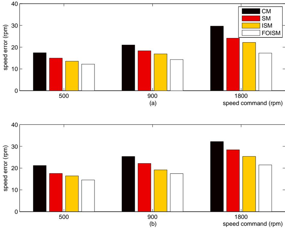
FIGURE 15. Experimental results of speed steady-state errors with different methods: (a) without load, (b) load applied
