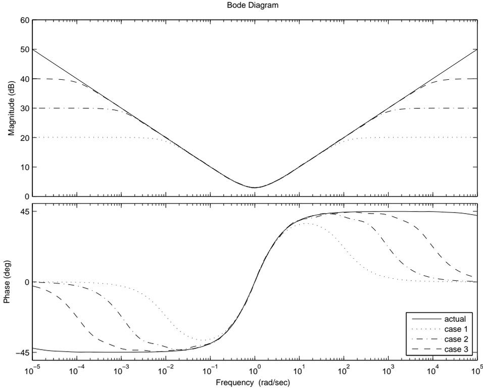
FIGURE 1. Frequency responses of the approximations to the transfer function  $s^{-0.5} + s^{0.5}$  with different transitional frequencies
