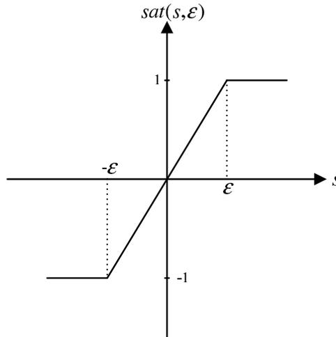
FIGURE 2. The diagram of the saturation function
