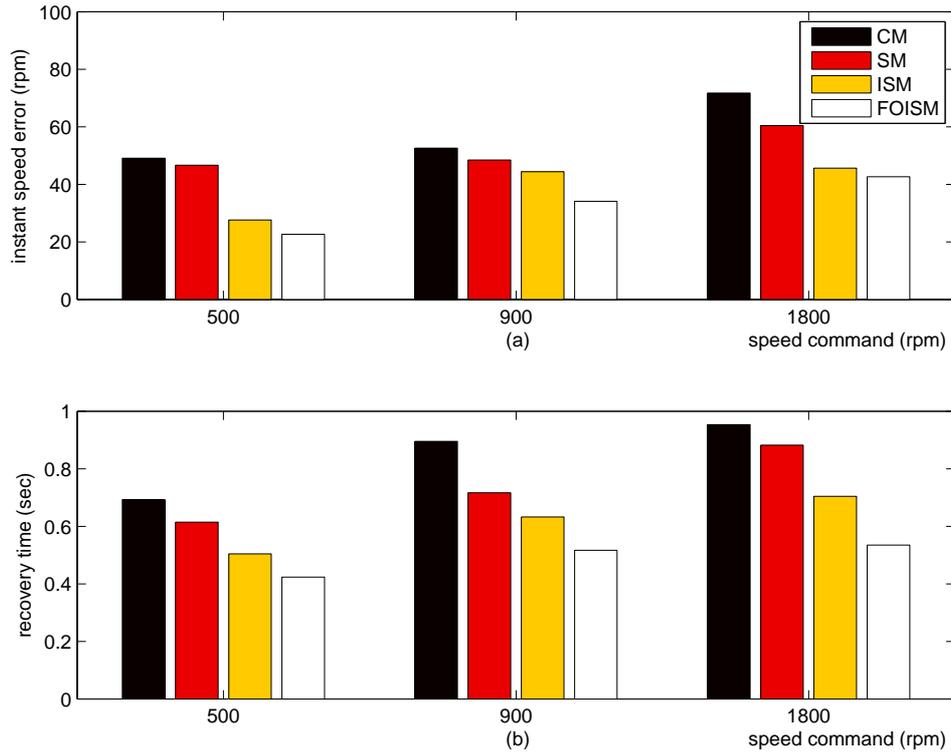
FIGURE 14. Experimental results of speed transient responses with load suddenly removed: (a) tracking error, (b) recovery time
