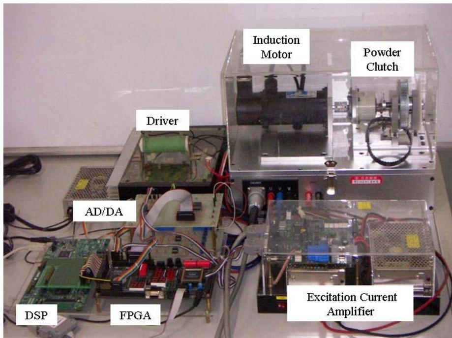
FIGURE 8. The experimental system setup
