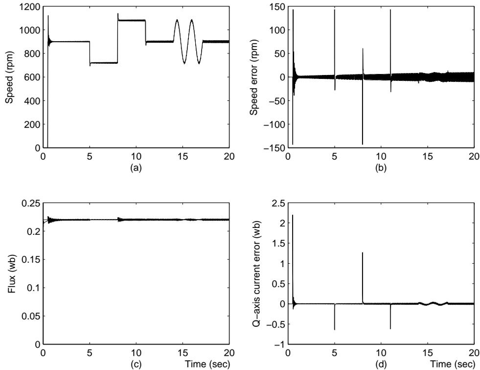
FIGURE 6. Simulation results corresponding to the ISM flux observer: (a) speed response, (b) speed error, (c) rotor flux, (d)  $q$ -axis current error
