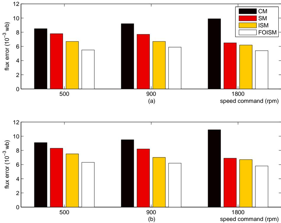
FIGURE 16. Experimental results of flux steady-state errors with different methods: (a) without load, (b) load applied
