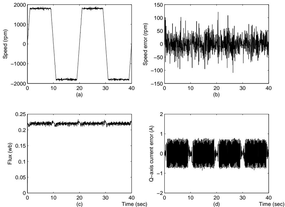
FIGURE 10. Experimental responses corresponding to the SM flux observer on  $\omega_{rm}^* = 1800$  rpm: (a) speed response, (b) speed error, (c) rotor flux, (d)  $q$ -axis current error
