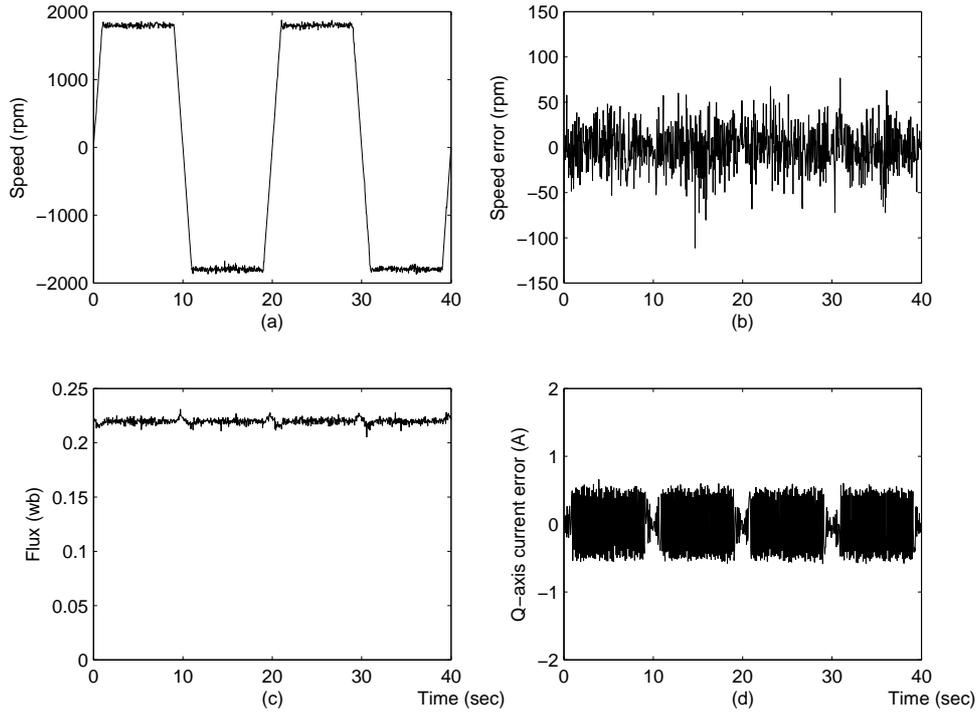
FIGURE 11. Experimental responses corresponding to the ISM flux observer on  $\omega_{rm}^* = 1800$  rpm: (a) speed response, (b) speed error, (c) rotor flux, (d)  $q$ -axis current error
