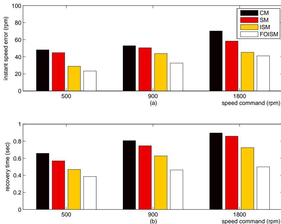
FIGURE 13. Experimental results of speed transient responses with load suddenly applied: (a) tracking error, (b) recovery time
