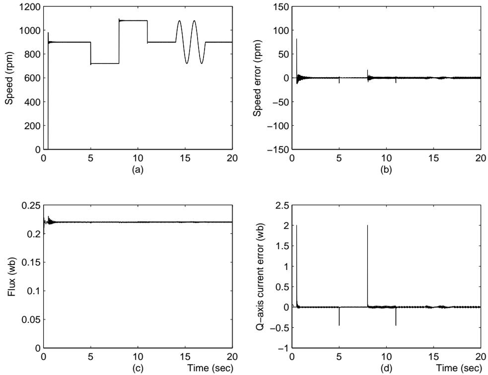
FIGURE 7. Simulation results corresponding to the FOISM flux observer: (a) speed response, (b) speed error, (c) rotor flux, (d)  $q$ -axis current error
