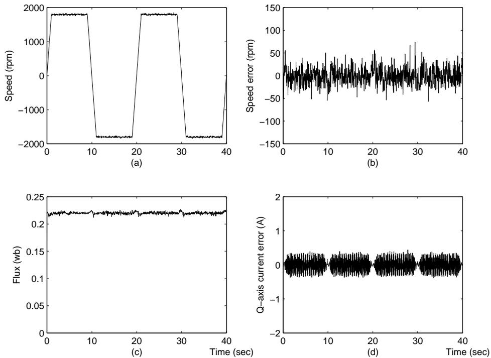
FIGURE 12. Experimental responses corresponding to the FOISM flux observer on  $\omega_{rm}^* = 1800$  rpm: (a) speed response, (b) speed error, (c) rotor flux, (d)  $q$ -axis current error
