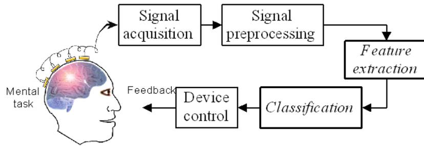
FIGURE 1. Basic five key steps in BCI (the feature extraction and classification steps are focused in this paper)
