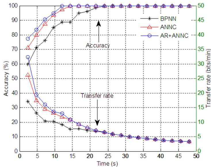
FIGURE 9. Classification accuracy and transfer rate obtained with BPNN, ANNC, and the ANNC with the AR model, averaged over all disabled subjects
