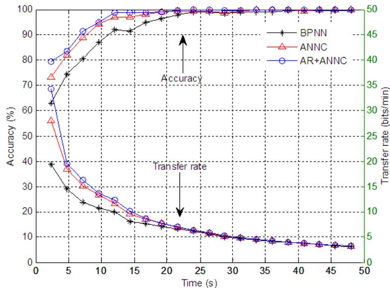
FIGURE 11. Classification accuracy and transfer rate plots obtained with BPNN, ANNC, and the ANNC with the AR model, averaged over all subjects
