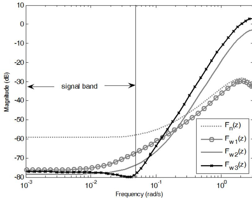
FIGURE 3. Bode plots of  $(NTF_1(z) - F(z) \times STF_2(z))$  matched by filters; parameter deviations  $\delta_a = \delta_b = 0.01$  in  $H_i(z)$  ( $i = 1, 2, 3$ )
