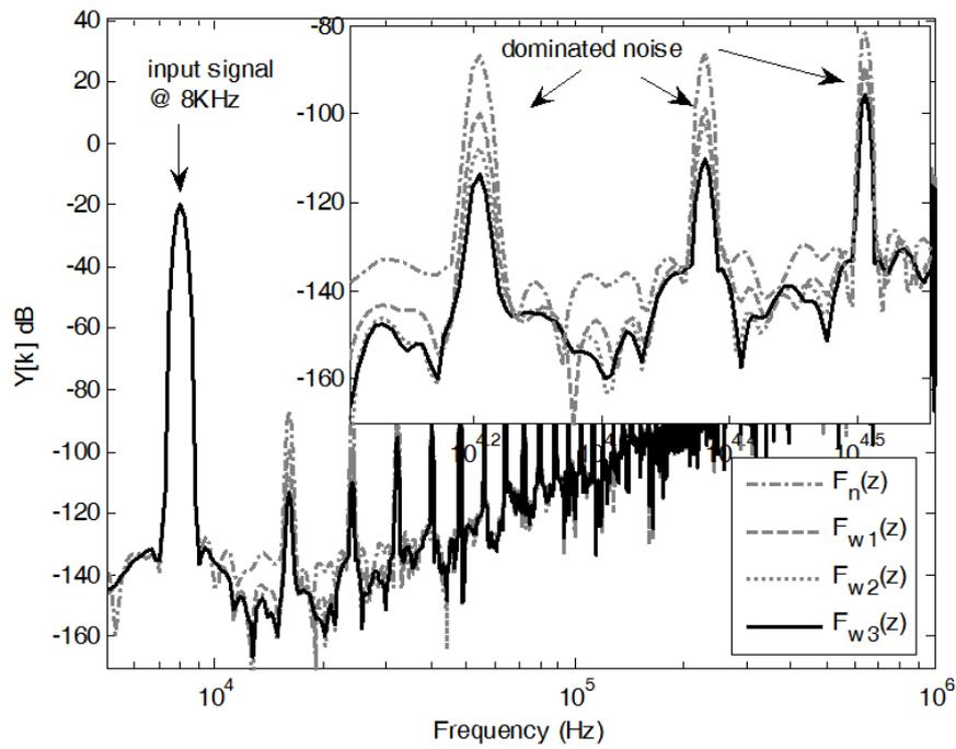
FIGURE 4. Power spectrum density of uncertain modulator matched by filters; parameter deviations  $\delta_a = \delta_b = 0.01$  in  $H_i(z)$  ( $i = 1, 2, 3$ )
