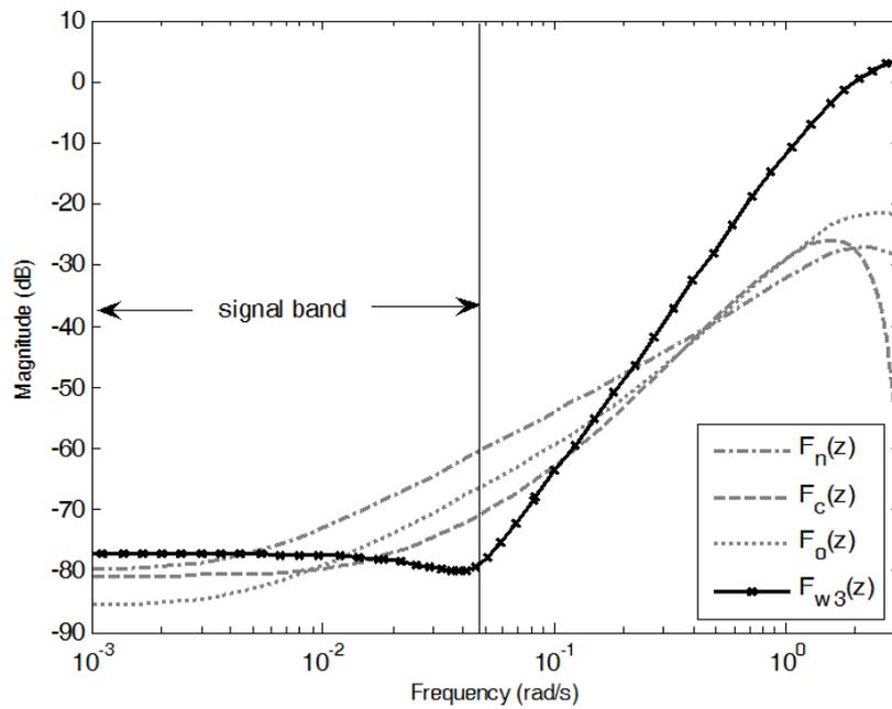
FIGURE 5. Bode plots of  $(NTF_1(z) - F(z) \times STF_2(z))$  matched by filters; parameter deviations  $\delta_a = \delta_b = 0.01$  in  $H_i(z)$  ( $i = 1, 2, 3$ )
