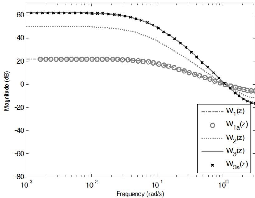
FIGURE 2. Bode plots of weighting functions
