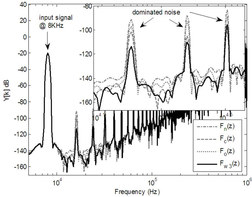
FIGURE 6. Power spectrum density of uncertain modulator matched by filters; parameter deviations  $\delta_a = \delta_b = 0.01$  in  $H_i(z)$  ( $i = 1, 2, 3$ )
