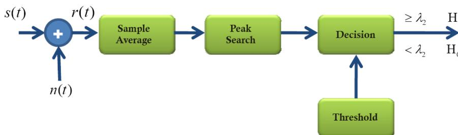
FIGURE 3. Block diagram of one-order cyclostationary detection [14]
