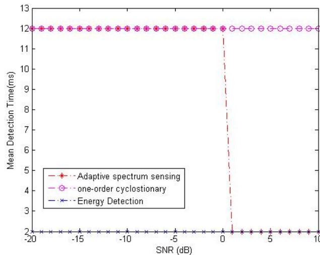
FIGURE 6. Mean detection time comparison of proposed adaptive spectrum sensing, one-order cyclostationary detector and energy detector
