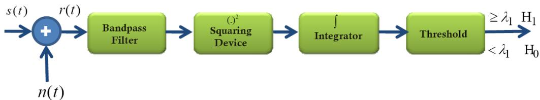
FIGURE 2. Block diagram of energy detection
