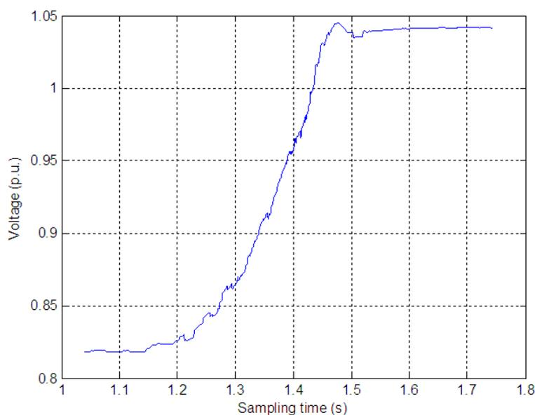
FIGURE 4. Measured load voltage profile
