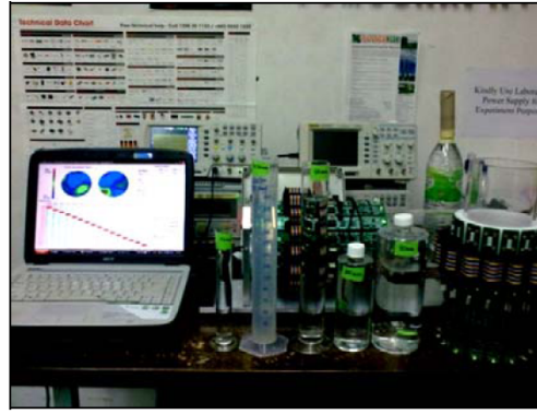
FIGURE 18. Portable ECT with bottle and test tube used to create phantoms inside the ECT sensor. Water is filled in the bottle and test tube, making up phantom of annular water flow.
