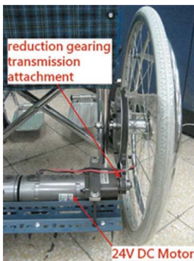
FIGURE 3. Motors, reduction gear and belt linkage to wheel
