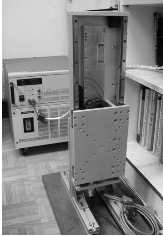
FIGURE 14. ILPMSM system vertical to the ground
