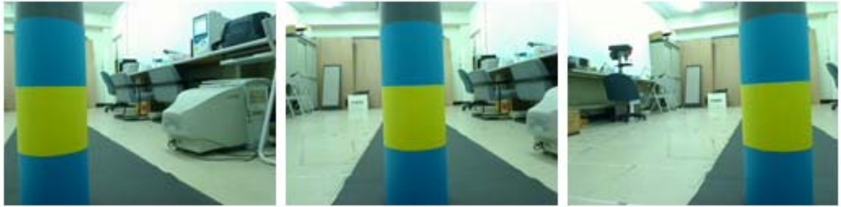
FIGURE 9. With the same distance from the robot to the landmark, (F_H, F_V) 's of the landmark at left, middle, and right positions of the frame are (86, 227) , (80, 219) , (87, 223) pixels, respectively.
