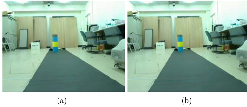
FIGURE 7. The landmark images with distances of: (a) 410cm and (b) 450cm. (F_H, F_V) are equal to (a) (14, 38), (b) (14, 38) pixels in the frame.
