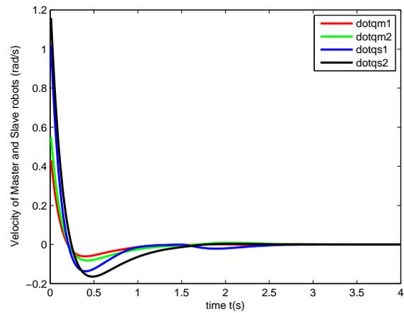
FIGURE 6. Master and slave joint velocities
