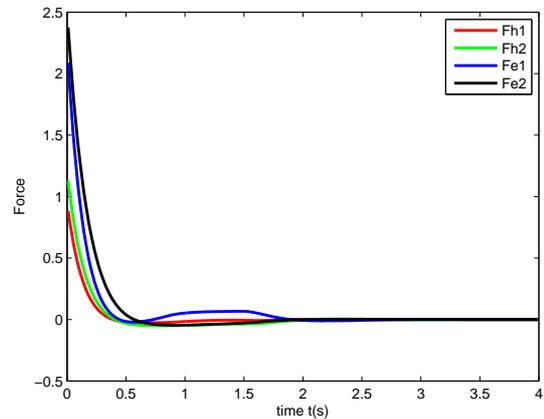
FIGURE 8. The human forces  $F_h$  and and the environmental force  $F_e$
