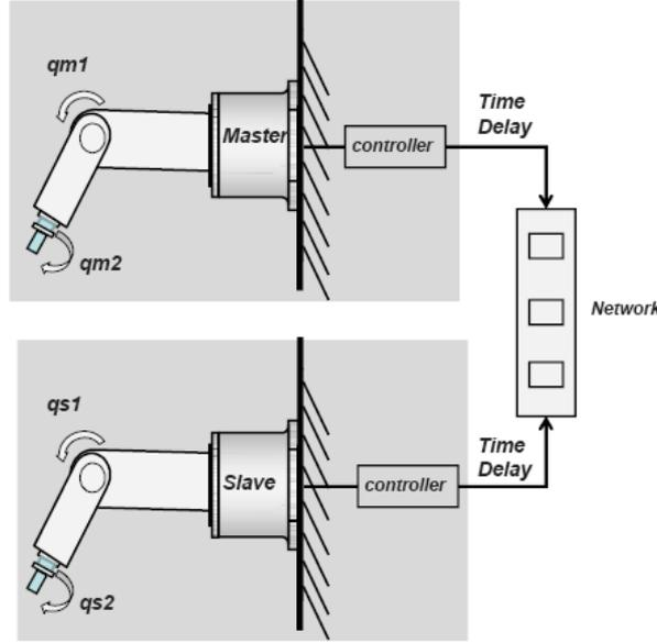
FIGURE 1. Motion synchronization of teleoperation system
