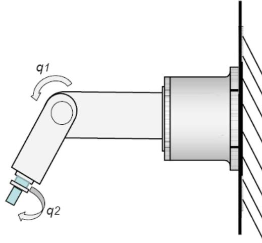
FIGURE 2. A 2-DOF robotic manipulator
