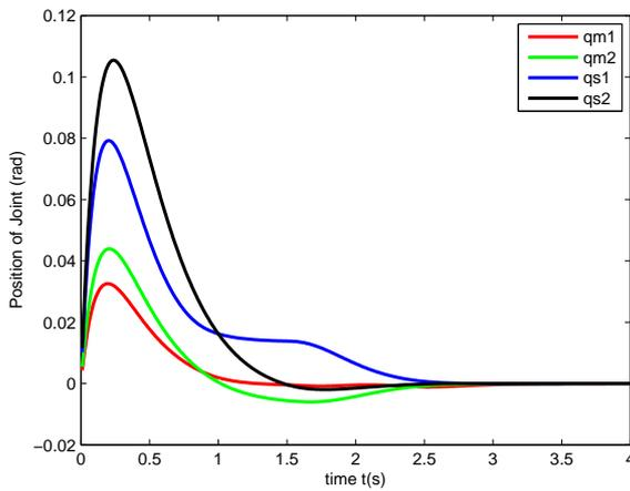
FIGURE 5. Master and slave joint positions
