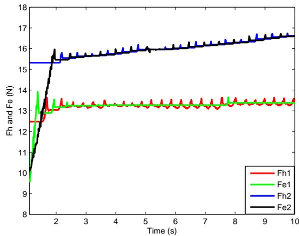
FIGURE 13. The human force  $F_h$  and the environmental force  $F_e$
