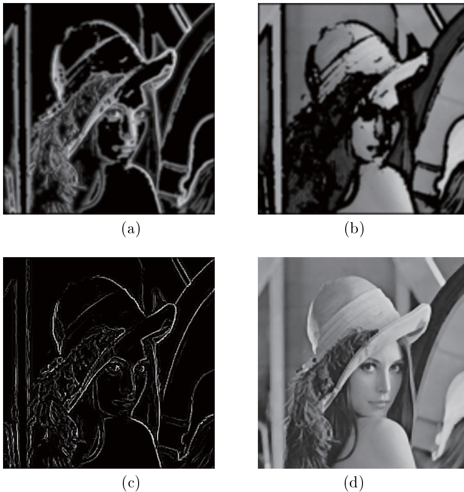
FIGURE 7. Result of edge detection for Lenna: (a) edge area, (b) non-edge area, (c) estimated high-frequency components, (d) augmented image
