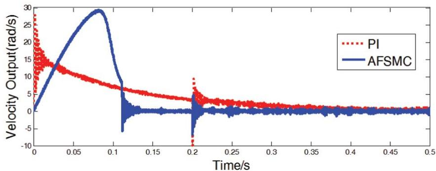
FIGURE 6. Comparison results of the velocity between AFSMC and PI controller under load disturbance
