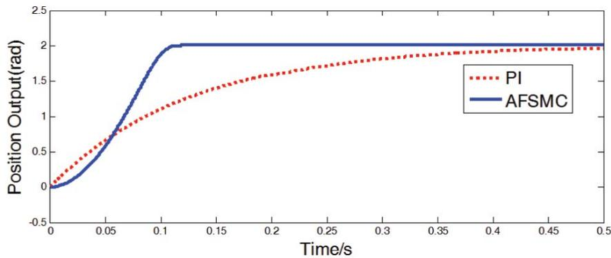
FIGURE 5. Comparison results of the position between AFSMC and PI controller under load disturbance
