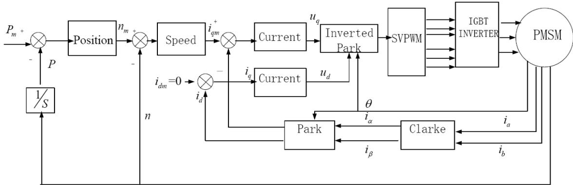
FIGURE 1. Control configuration of the PMSM system
