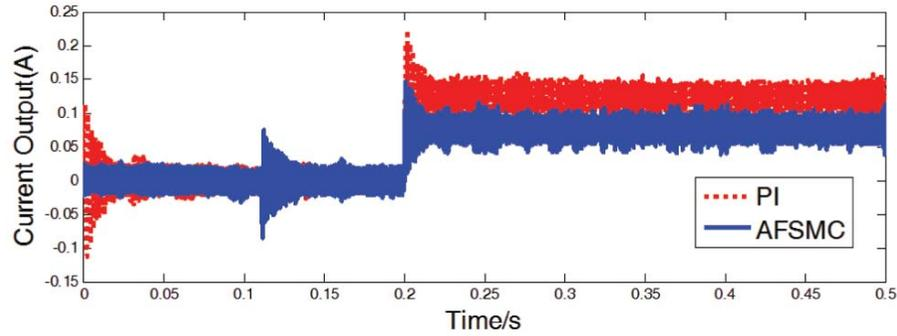
FIGURE 7. Comparison results of the current between AFSMC and PI controller under load disturbance
