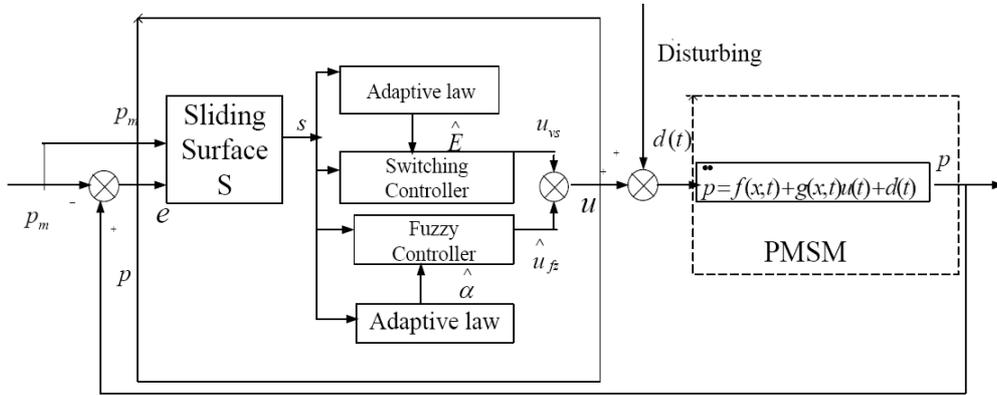
FIGURE 2. Block diagram of adaptive fuzzy sliding mode control system
