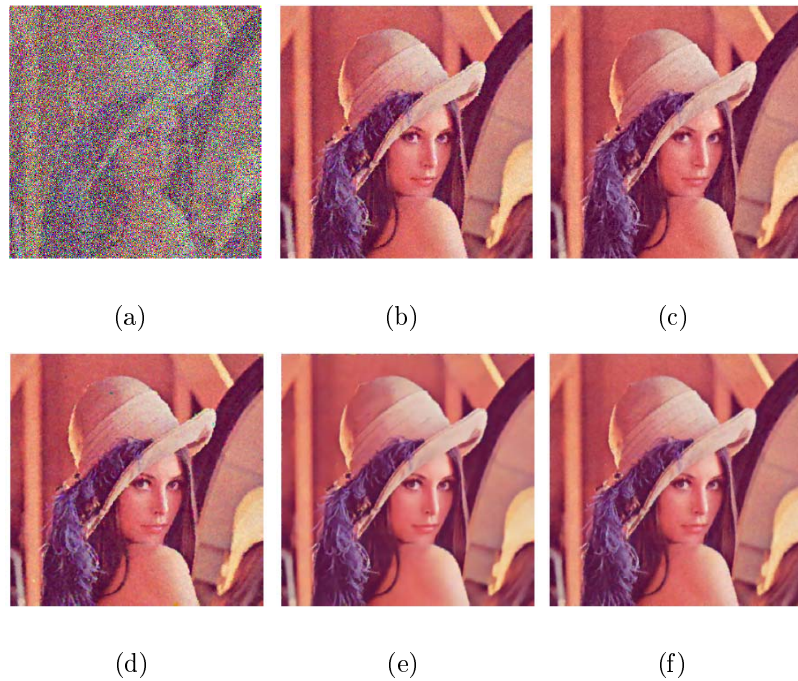
FIGURE 2. The filtering result of the Lena corrupted image. (a) Lena image is corrupted by Gaussian and impulse noise with \sigma = 10 and p = 70\% . (b) TP method [7]. (c) FTPID method [8]. (d) TV method [11]. (e) Modifying K-SVD [20]. (f) Proposed method.
