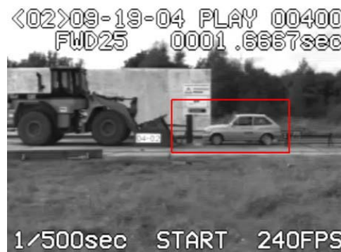
FIGURE 9. First frame used to describe the region of interest in the HFR video
