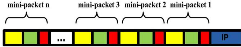
FIGURE 3. Mux-packet format
