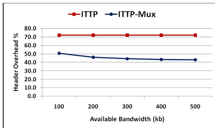
FIGURE 10. Header overhead
