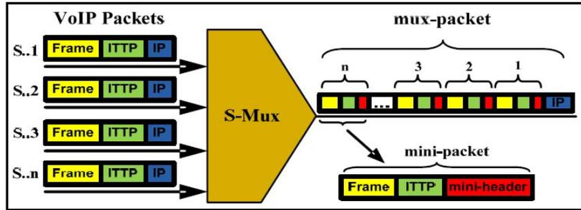
FIGURE 4. ITTP-Mux mechanism multiplexer (S-Mux)
