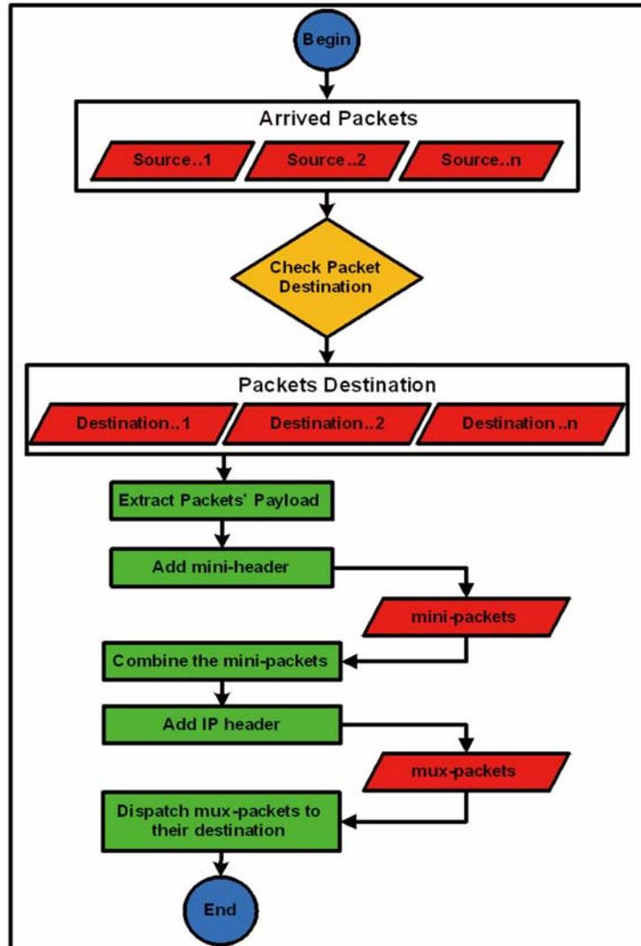
FIGURE 5. S-Mux internal process
