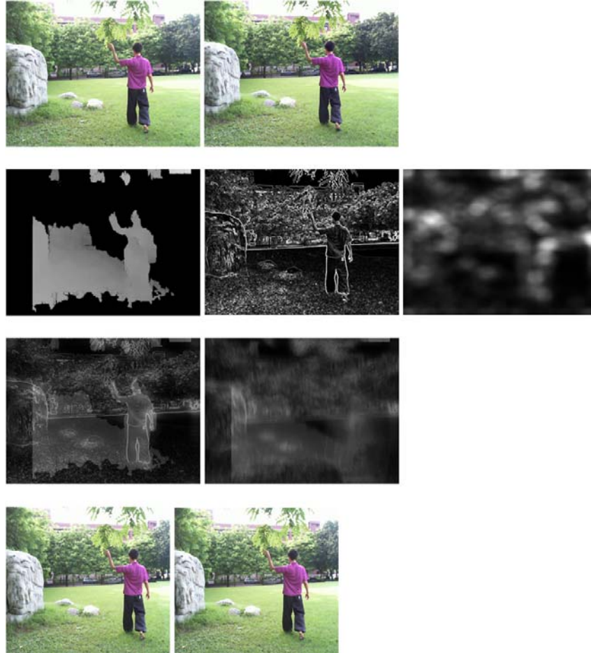
FIGURE 4. Original left-right images (the top row), the disparity map, gradient map and saliency map (the second row), the importance map and accumulated map (the third row), and resized results from left to right based on the importance map and the accumulated map, respectively (the bottom row)
