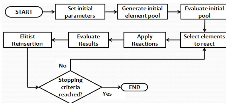
FIGURE 1. General flowchart of the chemical reaction algorithm
