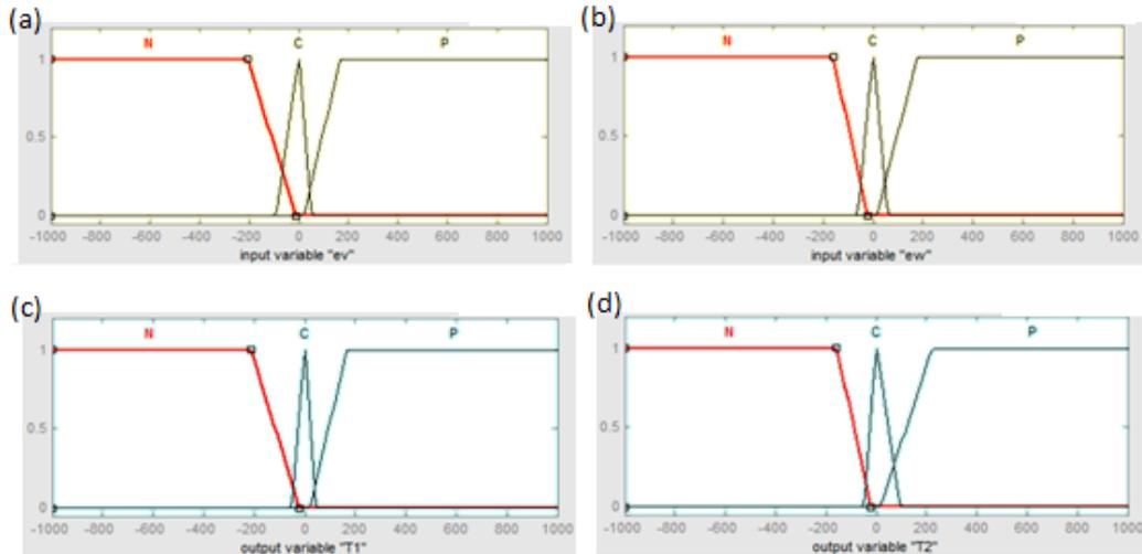
FIGURE 8. Resulting input membership functions: (a) linear and (b) angular velocities and output (c) right and (d) left torque
