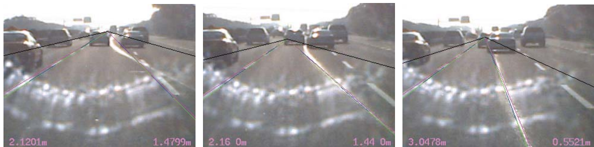
FIGURE 5. Wrong detection due to the extra liquid stripe on road surface
