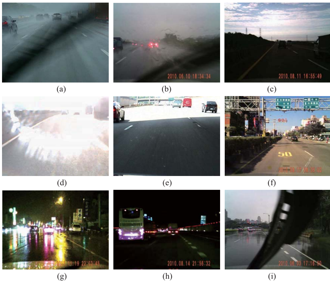
FIGURE 10. Image samples with various weather conditions and road-surface situations. (a) (b) Heavy rain. (c) (d) Glare from the sun. (e) (f) Cast shadow. (g) Light noise. (h) Night. (i) Double lane marks.
