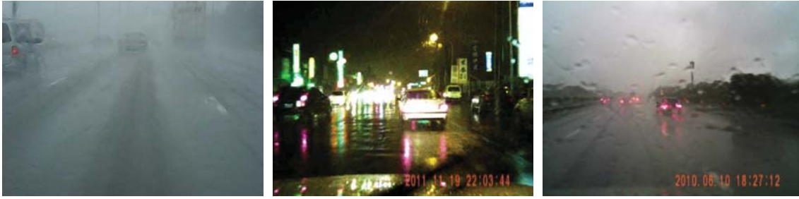
FIGURE 17. The very stubborn cases in which the lane marks are not detectable
