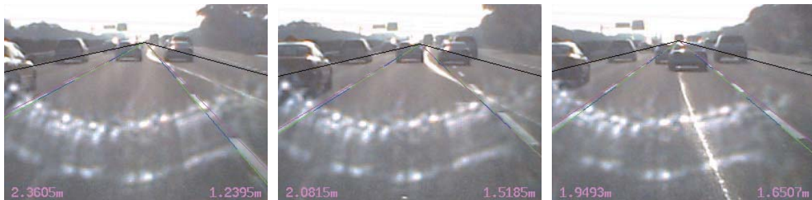
FIGURE 15. Lane marks are correctly detected from the liquid stripe
