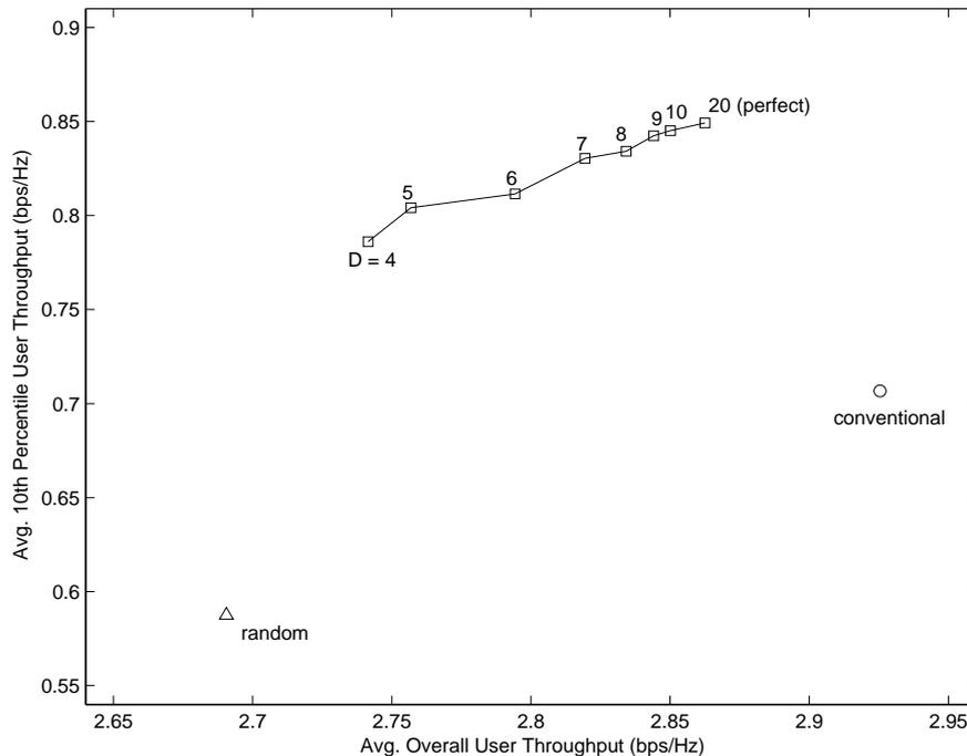
FIGURE 6. Average user throughput performance with the number of available link-gains for  $\epsilon = 0.05$
