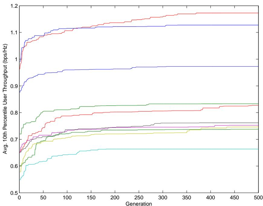
FIGURE 4. Convergence of the proposed scheme improving the performance of the 10th percentile user throughput for  $\epsilon = 0.05$
