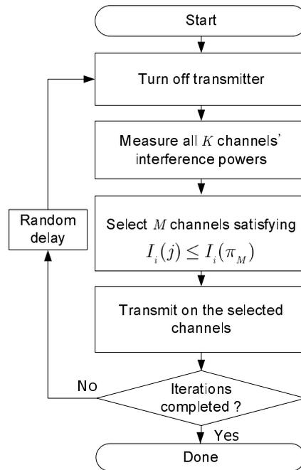
FIGURE 1. Flow chart of the conventional scheme
