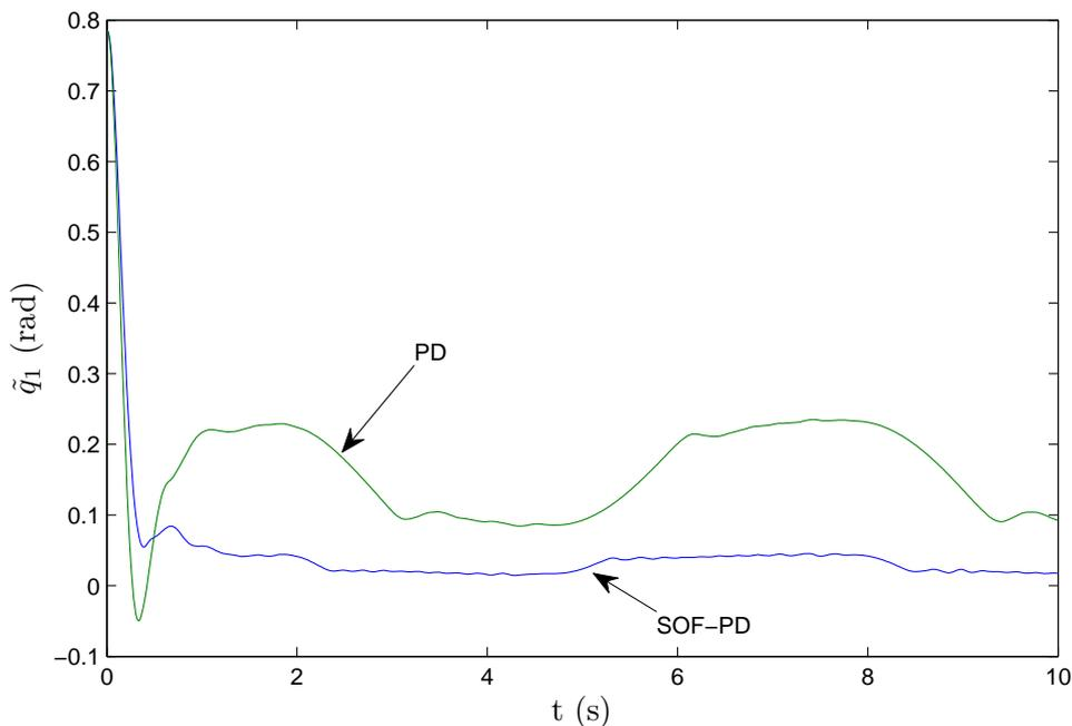
FIGURE 4. Tracking errors on  $q_1$
