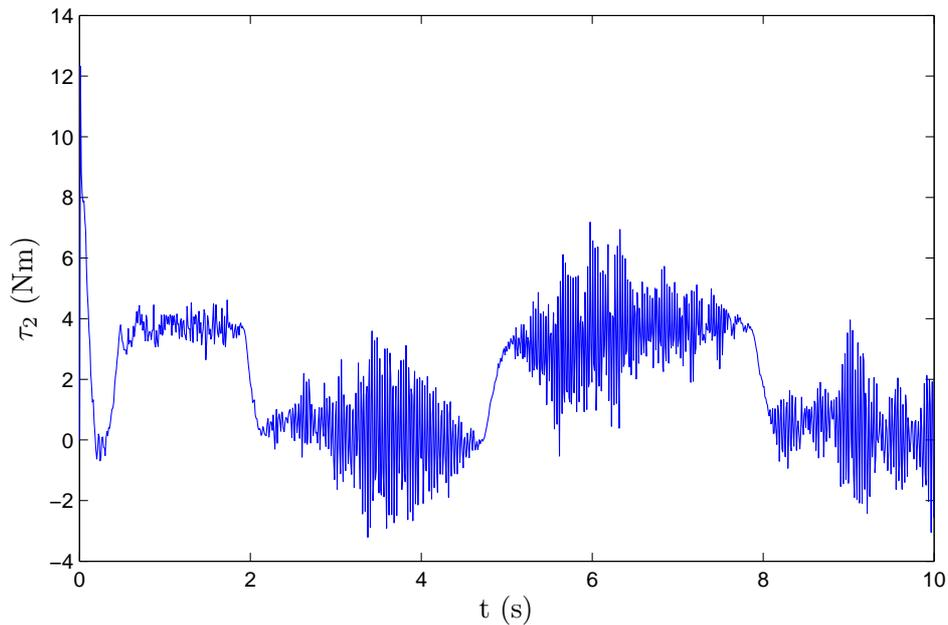
FIGURE 14. Torque  $\tau_2$  delivered with the new tuning of the SOF-PD
