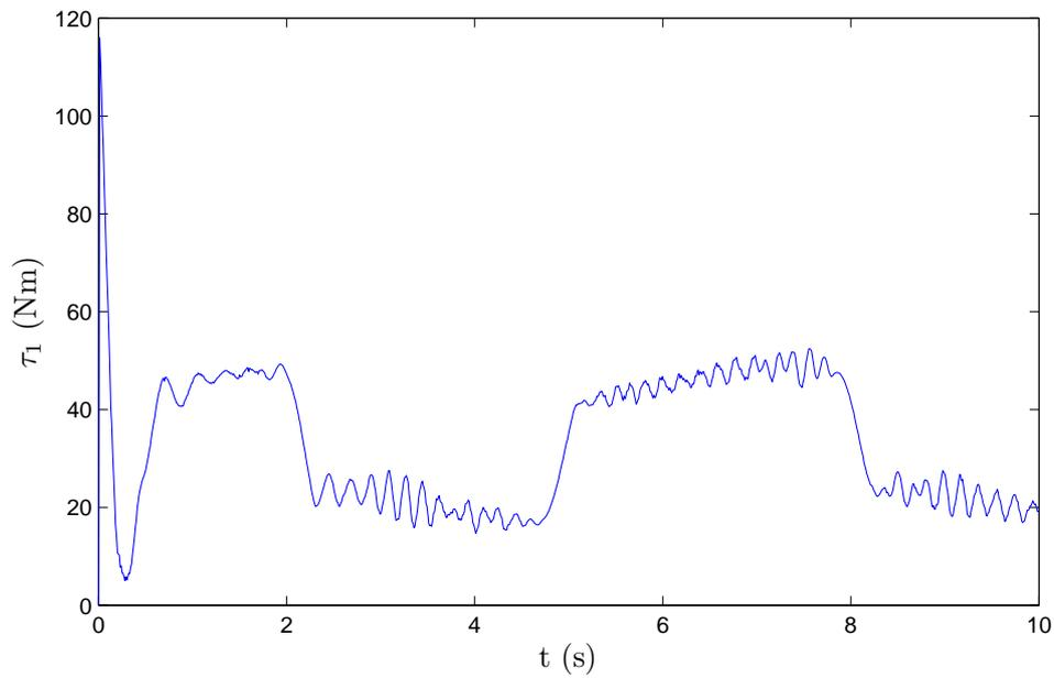
FIGURE 13. Torque  $\tau_1$  delivered with the new tuning of the SOF-PD
