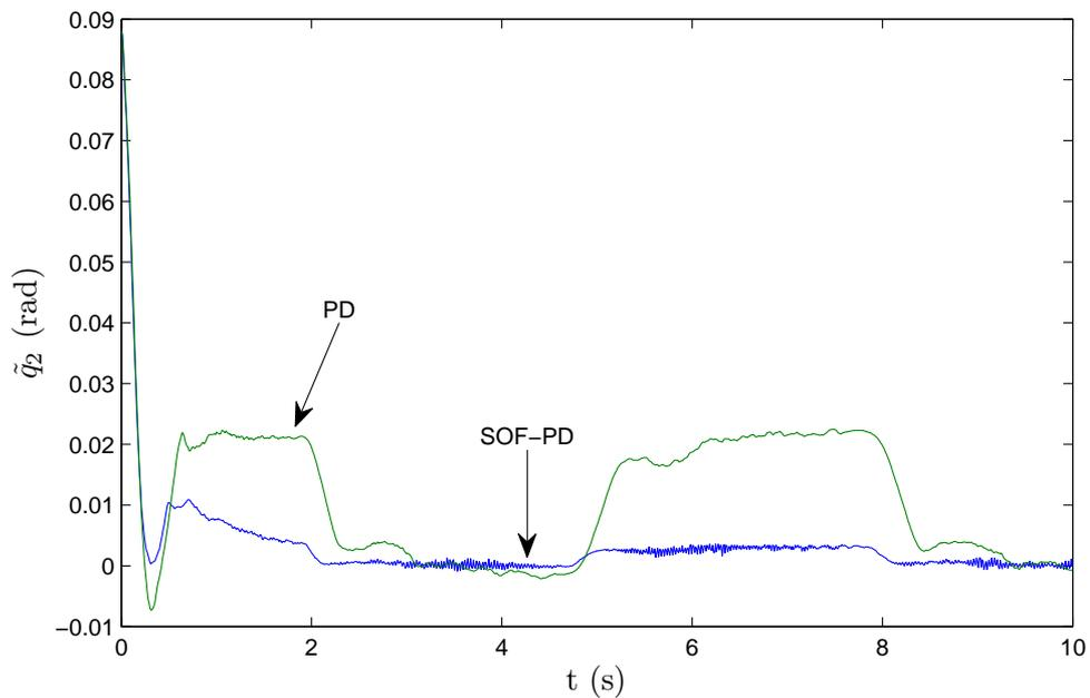
FIGURE 12. Tracking errors on  $q_2$  with the new tuning of the SOF-PD
