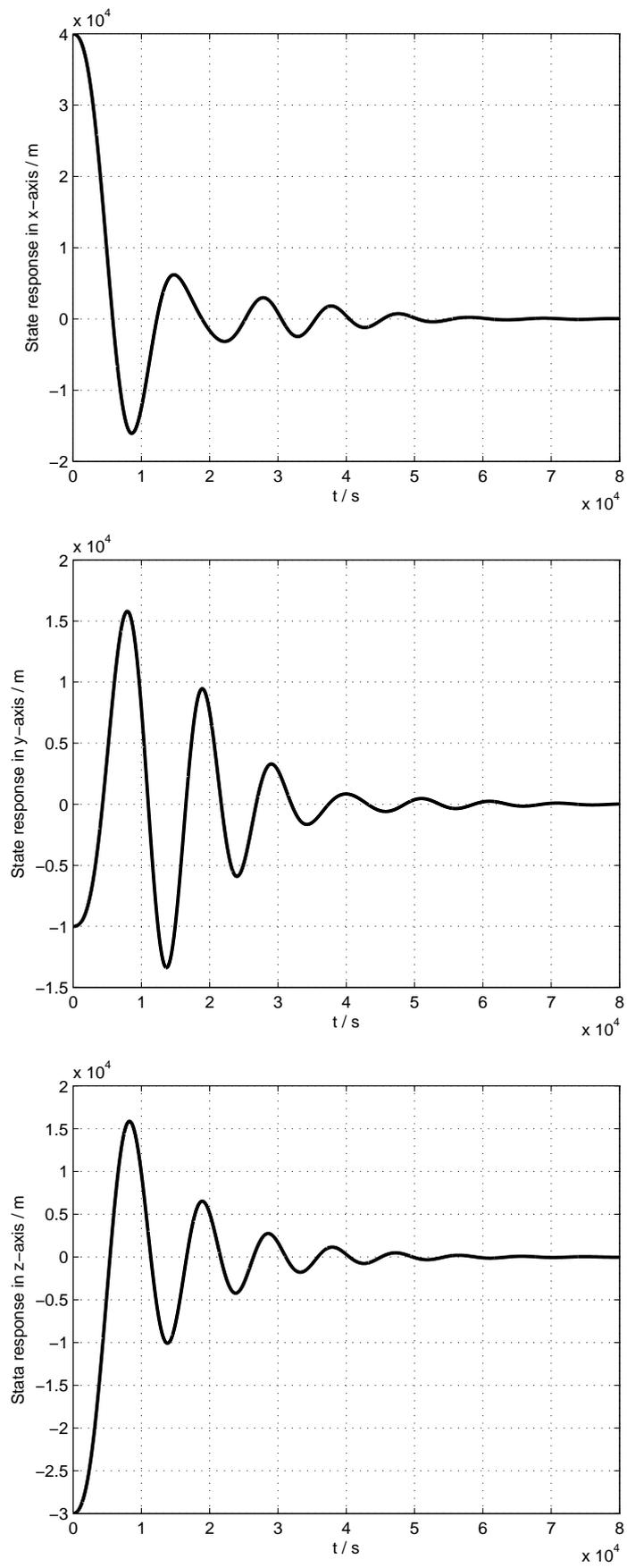
FIGURE 3. Relative position of the two spacecrafts
