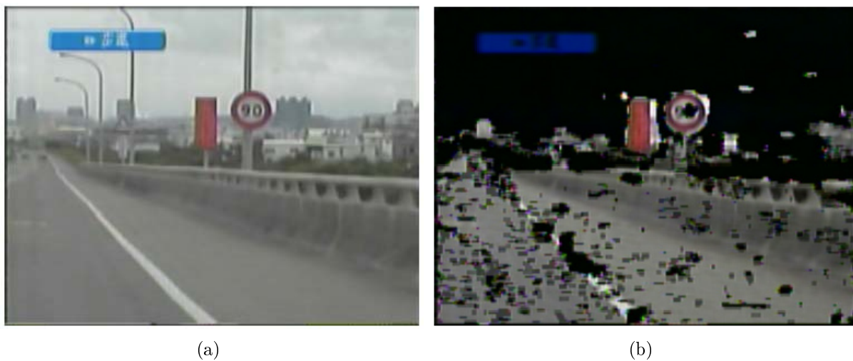
FIGURE 2. Segmentation result from HSI color space. (a) Original image. (b) Result of pan-red segmentation.
