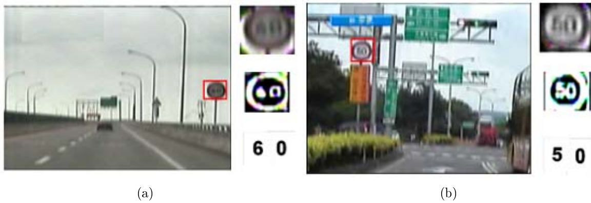
FIGURE 13. Two examples of recognition results under camcorder vibration. The right images are the detection results and the recognition results.
