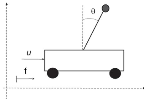
FIGURE 1. The inverted pendulum mounted on a cart
