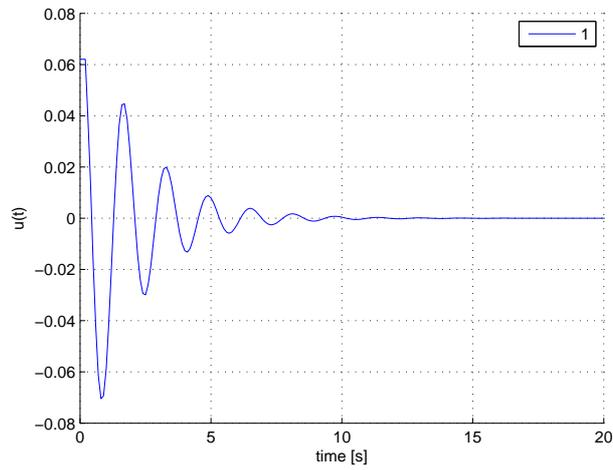
FIGURE 2. Time responses of the input  $u(t)$  without constraints
