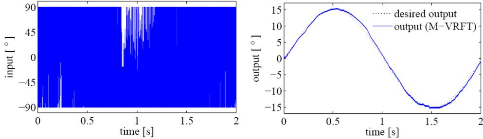
FIGURE 8. Control input and output using modified VRFT
