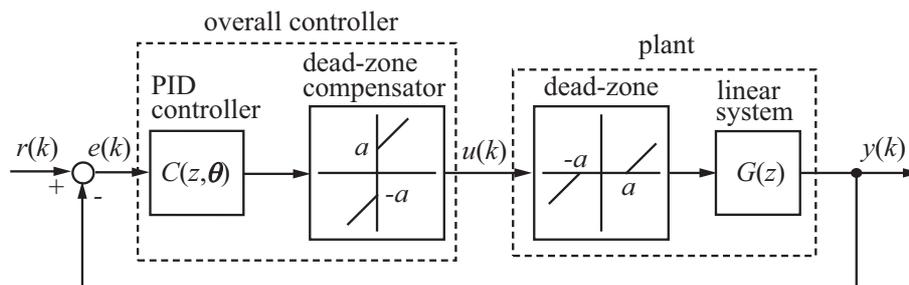
FIGURE 2. System configuration with dead-zone compensation
