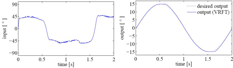
FIGURE 7. Control input and output using standard VRFT
