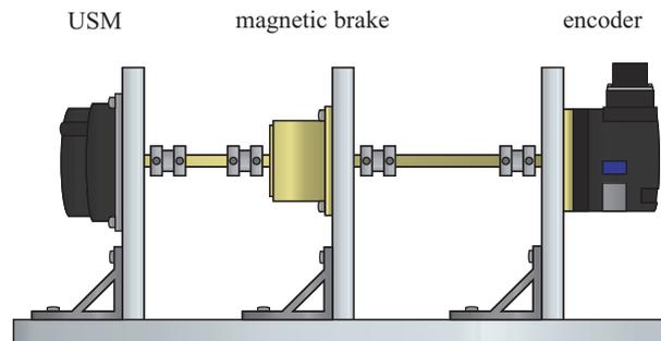
FIGURE 3. Experimental USM control system
