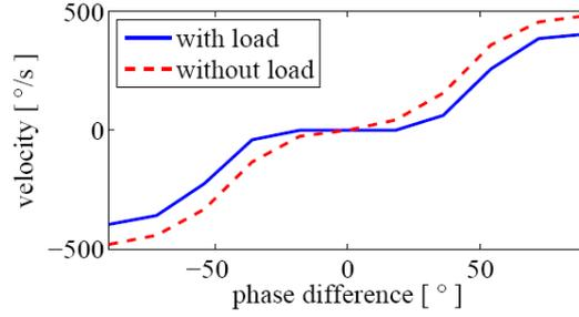
FIGURE 4. Dead-zone characteristics of USM
