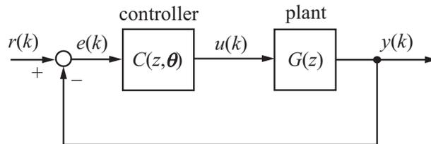
FIGURE 1. Standard feedback control system
