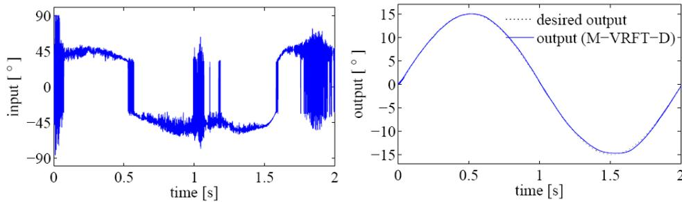
FIGURE 6. Control input and output using modified VRFT with dead-zone compensation
