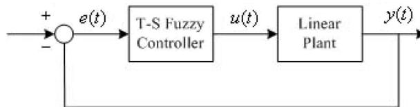
FIGURE 1. The control loop
