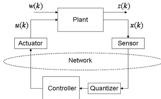
FIGURE 1. The structure of network control systems (1)
