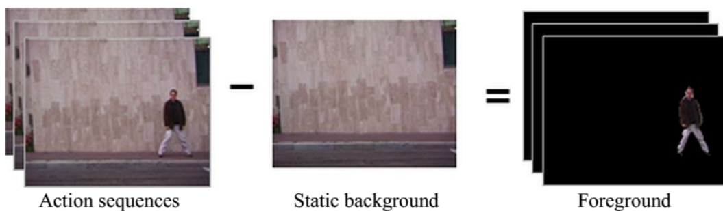
FIGURE 1. Simple illustration of foreground extraction
