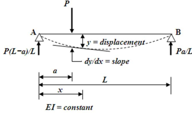
FIGURE 2. Beam “AB” subjected to a concentrated load
