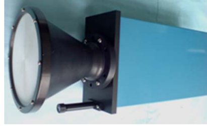
FIGURE 2. Photograph of the radar to measure the motion parameters of in-bore projectile
