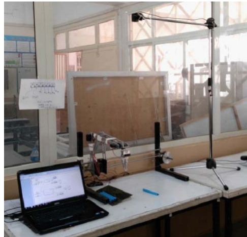
FIGURE 10. Experimental test rig with robot arm in home position
