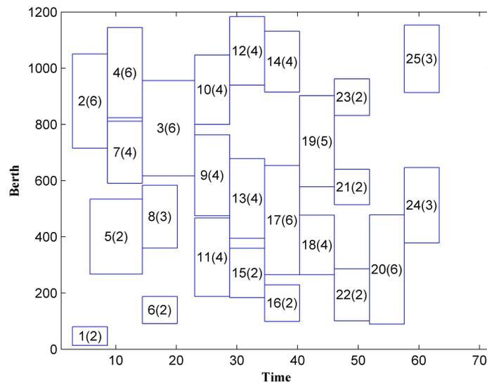
FIGURE 1. An optimal BCAP solution of an instance with 25 vessels
