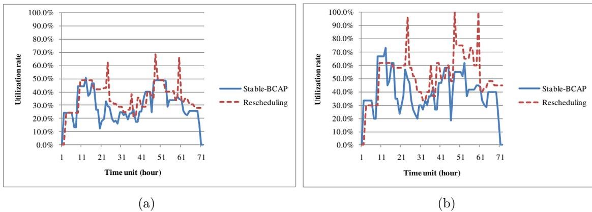
FIGURE 5. Comparison of utilization rate for berths and quay cranes ( $V = 22$ ): (a) utilization rate of berths and (b) utilization rate of quay cranes
