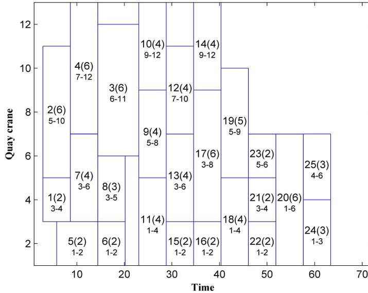
FIGURE 3. The quay crane allocation result for an instance with 25 vessels
