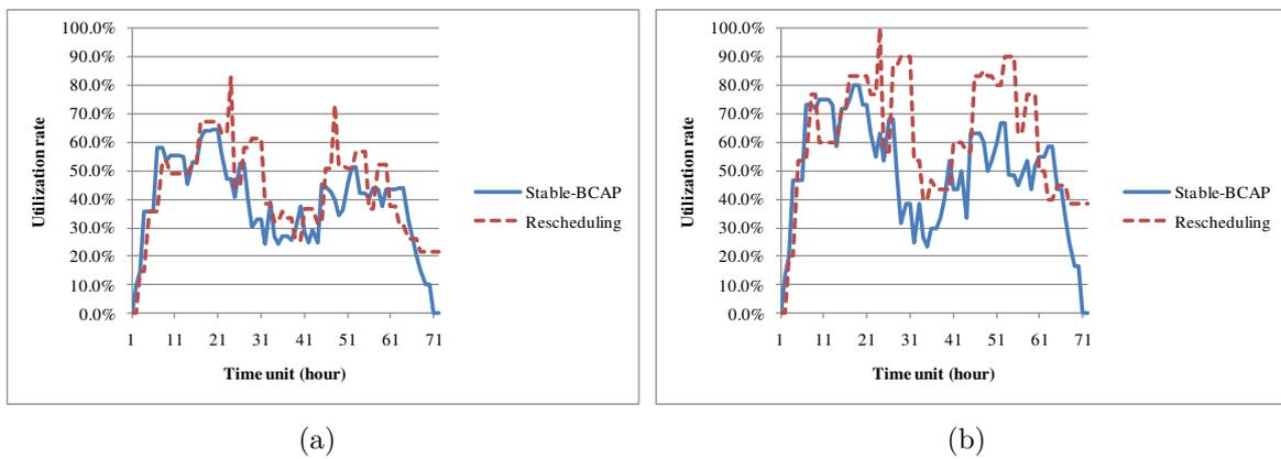
FIGURE 6. Comparison of utilization rate for berths and quay cranes ( $V = 25$ ): (a) utilization rate of berths and (b) utilization rate of quay cranes
