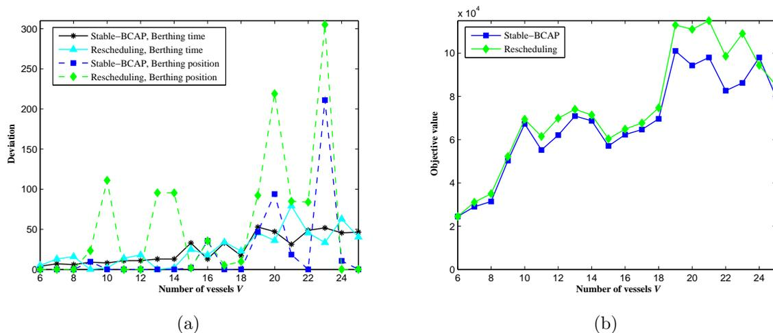
FIGURE 4. Comparison between Stable-BCAP strategy and rescheduling method: (a) deviations from initial scheduling and (b) objective values
