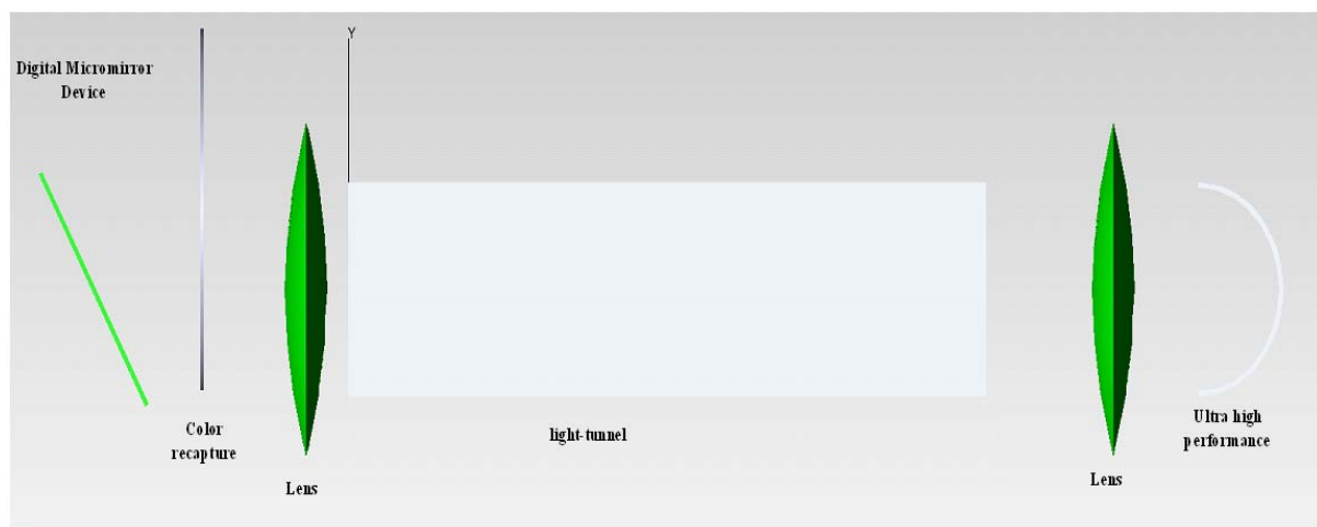
FIGURE 1. The traditional DLP optical engine
