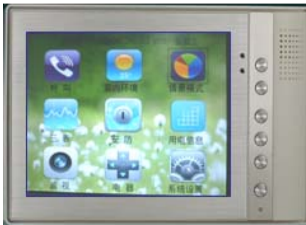
FIGURE 3. Smart home control unit
