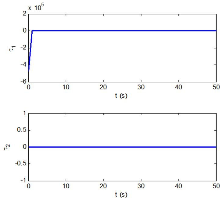
FIGURE 9. Surge force and yaw moment in stabilization case
