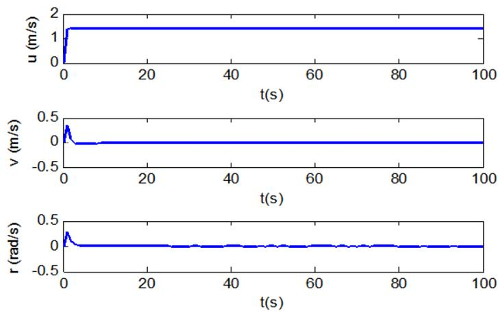
FIGURE 2. Velocity of surge, sway and yaw in straight-line case
