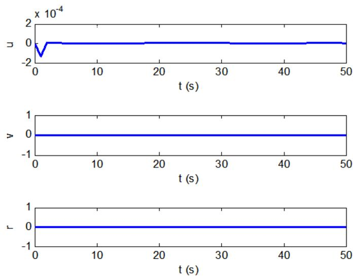
FIGURE 8. Velocity of surge, sway and yaw in stabilization case
