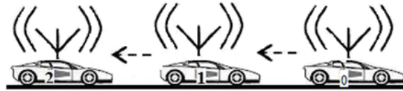
FIGURE 2. Communication network in a platoon of vehicles
