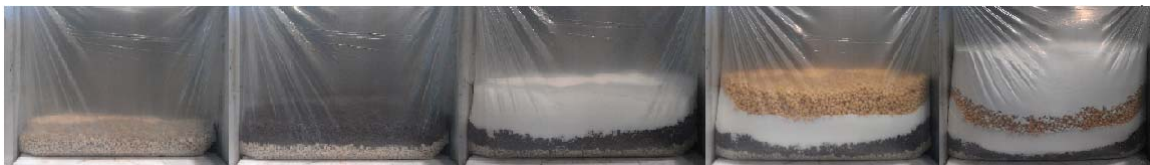
FIGURE 7. Height variation of material pile in multi-variety material batching process
