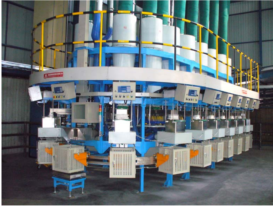
FIGURE 4. Schematic diagram of multi-station weighing and batching system
