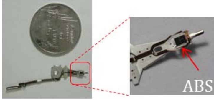
FIGURE 1. Air bearing surface on HGA and the size of a one-Thai baht coin
